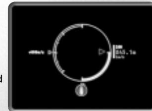
The left side of the reticle is the speed display. In conventional flight you can see your speed in meters per second to the left of the center. The orange arc displays your speed graphically, with the small orange triangle marking your set speed.
